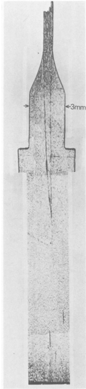
Figure 5 Longitudinal section of a specimen which failed in a conventional tensile mode. Note the “tram-lines”, terminating within the specimen shoulders (composite micrograph).
